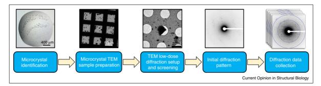
Flow diagram for MicroED data collection protocol. Source: Adapted from Ref. [47°].
